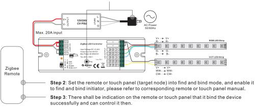
Note: Make sure the device and the remote or touch panel already added to the same Zigbee hub.
