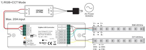
Note: please make sure the dial switches are at position for RGB+CCT mode as shown in above diagram. 2) RGBW Mode
