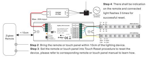
**Note:** Make sure the device already added to a network, the remote added to the same one or not added to any network.
