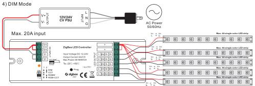
Note: please make sure the dial switches are at position for DIM mode as shown in above diagram.
