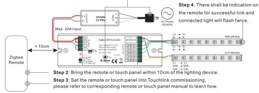
Note: 1) Directly TouchLink (both not added to a ZigBee network), each device can link with 1 remote.
