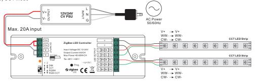
Note: please make sure the dial switches are at position for CCT mode as shown in above diagram.
