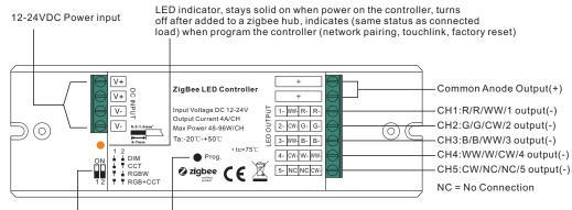
Dial switch for device mode selection, DIM, CCT, RGBW and RGB+CCT 4 modes are available, factory default is RGB+CCT mode
