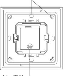
Battery: CR2430 <sup>I</sup> Before the first use, please open the battery cover and remove the protective film
