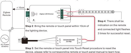
**Note**: Make sure the device already added to a network, the remote added to the same one or not added to any network.
