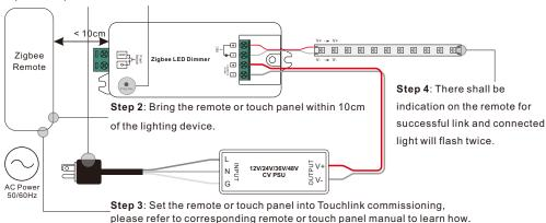
Note: 1) Directly TouchLink (both not added to a ZigBee network), each device can link with 1 remote.
