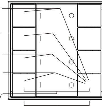
Network pairing mode: click both buttons 3 times to set the remote into network pairing mode (the remote should not belong to any gateway network).
