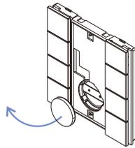
3) Remove the battery insulator
