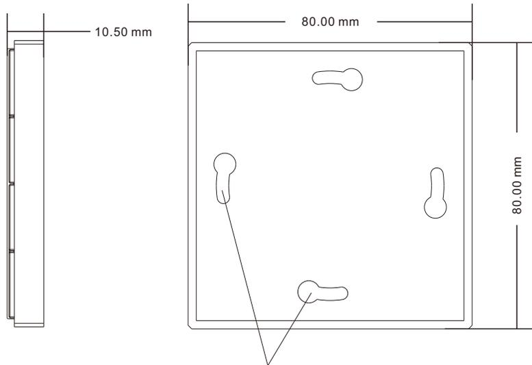
The switch can be fixed on the wall with 3M glue or screw.
