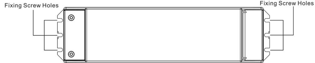
**Note:** when mounting the driver, please choose any one of the three fixing screw holes to fix with a screw at each end.
